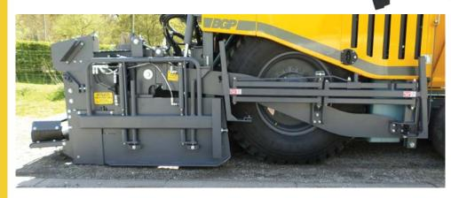
Travelling multi sensor levelling system with folding hardware ensures precise and accurate control takes only minutes to install and set up.
