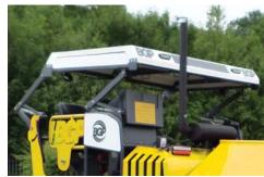
D Ease of access for the purpose of manual operation of key paving functions. Lockable side panels provide full access when needed.
