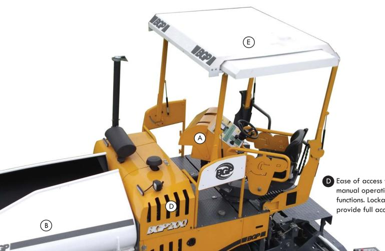
E Heavy duty fibreglass canopy folds easily for transportation. The canopy is equipped with extending sections to offer operator protection when the operators console is positioned outboard.
