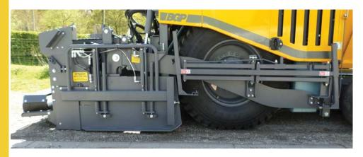
Travelling multi sensor levelling system with folding hardware ensures precise and accurate control takes only minutes to install and set up.
