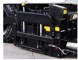
Optional switch controlled Hydraulic Raise Lower screed adjusting side plates makes light work of maintaining a precise and neat end joint and enhances operator safety during live traffic situations.
