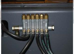
Assured and precise lubrication comes as standard on the MDTV screed unit. Automatic centralised time scheduled greasing on the tamper and vibrator circuits provides the precise amount required at the correct working intervals.
