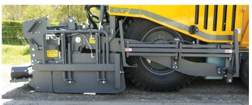
Travelling multi sensor levelling system with folding hardware ensures precise and accurate control takes only minutes to install and set up.
