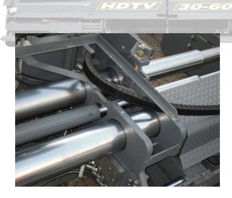
Twin - Large diameter - Wide centres screed extensions support tubes provide extension stability whilst maintaining uniform screed extension alignment.
