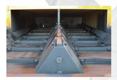
Deep conveyor tunnel depth and proportional conveyor speed ensures high volume and precise material throughput is maintained. Utilising Hardox conveyor floor wear material and adjustable conveyor side and centre guards optimises conveyor wear component life.
