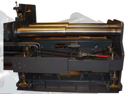
Assured and precise lubrication comes as standard on the HDTV screed unit. Automatic centralised time scheduled greasing on the tamper and vibrator circuits provides the precise amount required at the correct working intervals.
