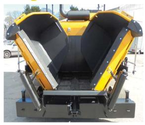
Independent switch operated hinged hopper front apron plate prevents material spillage out of the front receiving hopper, benefitting overall machine screed level control whilst enhancing operator safety by significantly reducing manual clearing of material residue in the front receiving hopper area. LED safety lighting system ensures safe entry - exit from the delivery truck.
