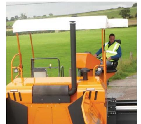
**A** Latest generation console with colour LCD display (with automatic adjustment for sunlight) has clearly laid out switch gear in logical and ergonomic positions which for the operator soon become second nature.
